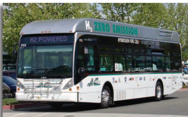
AC Transit's Hydrogen Fuel Cell-Hybrid Electric Drive Bus
