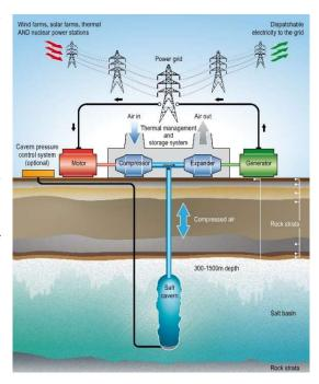
suit a vast range of applications / use cases, concurrently delivering grid stability based on real inertia. With the potential to store the entire continent's energy requirements for over a week, global potential is greater still. In the future, Storelectric will further develop both these and hybrid technologies, and other geologies for CAES, all of which will greatly improve storage cost, duration, efficiency and global potential.
